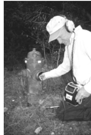
Finding leaks in rural and remote areas is another matter. Some techniques are: visual inspection of lines (on foot), testing unusual standing water for chlorine or fluoride, investigating indicative vegetation (like cattails or unusually green) near water lines. Leak
